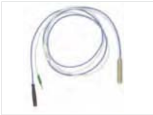
Art.-no. 520 071 Monopolar stimulation adaptor for disposable electrodes for adaptation to MS probes or MS instruments to DNS stimulation cable. 2 cables, one cable with 1 mm connector green for disposable neutral electrode; one cable with 1.5 mm touchproof connector black. Delivered non-sterile, autoclavable. Cable length 0.7 m.
