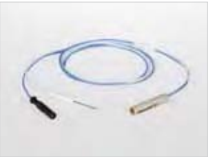
Art.-no. 520 070 Monopolar stimulation adaptor with needle electrode for adaptation to MS probes or MS instruments to DNS stimulation cable. 2 cables, one cable with needle L = 20 mm, neutral white; 1 cable with 1.5 mm touchproof connector black. Delivered non-sterile, autoclavable. Cable length 0.7 m.
